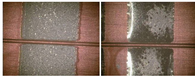
Figure 6: Solder Paste a) after printing and b) after reflow
